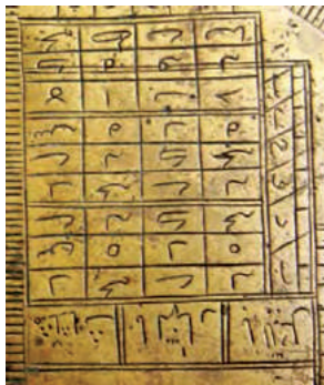
Fig. 10. Table of Triplicities engraved upside down (on the right there is a fragment of the shadow square with numbers 2, 4, 6, 8, 10, 12). Detail of Fig. 9.
